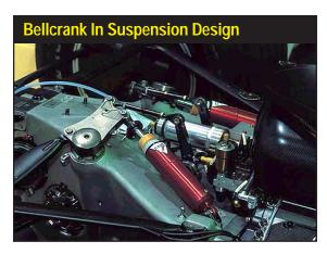
that use separate bellcranks for the spring and damper. FastLapSim supports none, single-, and dual-bellcrank designs.
