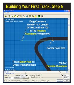
Now repeat the procedures performed in Step 5 on Corner Point #1. With the Selection Tool activated, highlight the Corner Point and extend the reverse curvature handle (with the blue square) to a length of 700, or enter 700 directly in the Reverse Curvature Scale box. Click on the Match Fwd button to align the Corner Point direction with the next Corner Point (Point #2). Your track should look similar to this photo.
