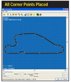
Continue placing Points, in order, until you have created Corner Points at all measured locations on the track. The track should look similar to the Track Map, except that the corners will be too "square." If, while you are placing points, you click in the wrong location, simply click the Undo Tool and re-place that point. When you have placed all Corner Points, deselect the Build Track Tool by clicking on the Selection Tool. Your Track Editor screen should look like this.
