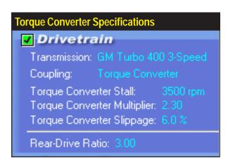
When any torque converter is selected, the Stall Rpm, Torque Multiplier, and Slip percentage fields become active in the DRIVETRAIN category. Use FastLapSim built-in selections or DirectClick™ any data field and enter custom values.
