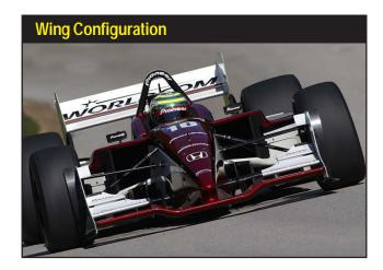
The wing models used in FastLapSim include end plates and Gurney flaps. In addition, the simulation includes chord-angle modeling. This is a measurement of the shape of wing surfaces and provides an indicator of the ability to produce lift with a zero attack angle. In FastLapSim the chord angle is set to zero degrees; lift is produced only when the angle of attack is greater than zero.
