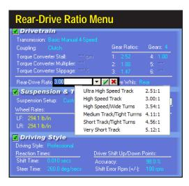
The Rear-Drive Ratio is the numerical gear ratio of the front or rear driving axle, depending on whether the vehicle is front- or rear-wheel drive. This ratio indicates the number of turns the driveshaft (or pinion gear) rotates for each revolution of the rear wheels.
