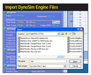
FastLapSim will directly import DynoSim engine files. To load a DynoSim test engine, select Import DynoSim Engine File from the Engine menu. A fileopen dialog box allows you select any DynoSim file on your system. The default location for DynoSim engine files is C:\DynoSim\EngineFiles (.DYN)
