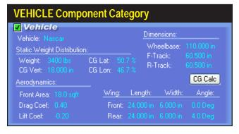
The domestic, import, and race Vehicle component menus contain predefined vehicle specifications that you can instantly select and use in a simulation. In addition, you can modify any of these built-in vehicle combinations with custom wheelbases, weights, frontal areas, and other component specifications.
