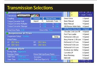
FastLapSim offers an extensive list of Manual and Automatic transmissions for both domestic and sport-compact applications. It is also possible to DirectClick™ on any DRIVETRAIN data field and enter custom transmission specs. When a transmission selection is made, the *Number Of Gears* and the *Gear Ratios* are loaded into DRIVELINE component fields.
